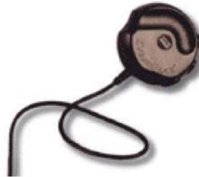
Cyberpuck for motion control in 6 degrees of freedom
